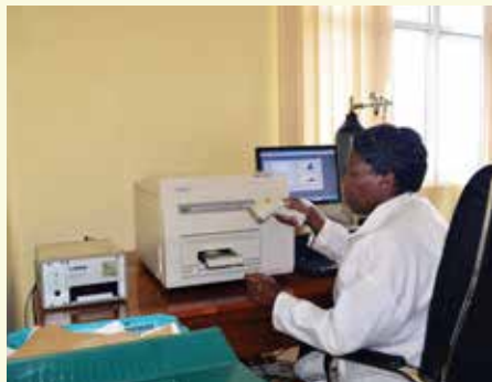
Dose reading on Thermoluminescent Dosimeter at Dosimetry Laboratory
