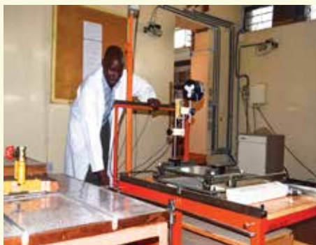
Survey Meter Calibration at Secondary Standard Dosimetry Laboratory (SSDL)
